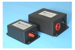
The Model 610 and 650 Current Shunts are specifically designed to operate with the Model 6000A Precision Phase Meter. These shunts are frequency tuned to have negligible phase shift (less than  $\pm$  5m°) at 50/60Hz making them ideal for line frequency applications. They can also be idealized for other frequencies as specified by the user. Consult factory for details.
