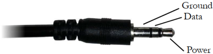
Figure 8: 3.5 mm Stereo Plug Wiring
