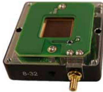
Figure 3-15. Align Pass-Thru Board in Sensor Housing
