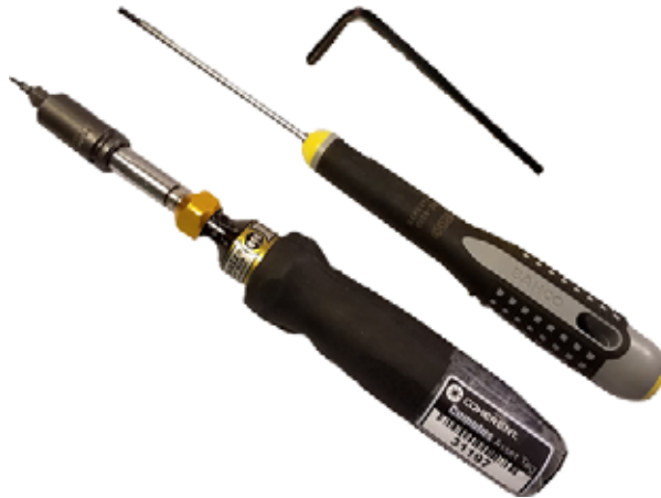
Figure 3-2. Tools Required to Disassemble the Sensor
