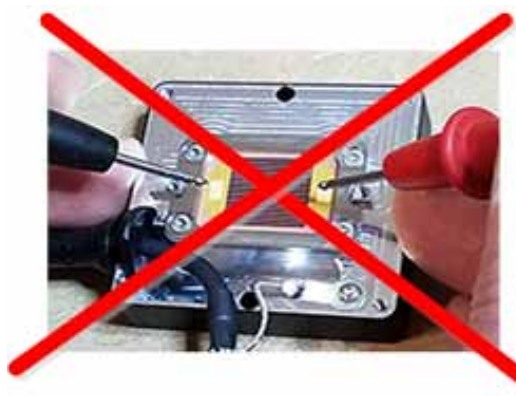
Figure 2-1. WARNING: Do NOT Probe the Sensor!
