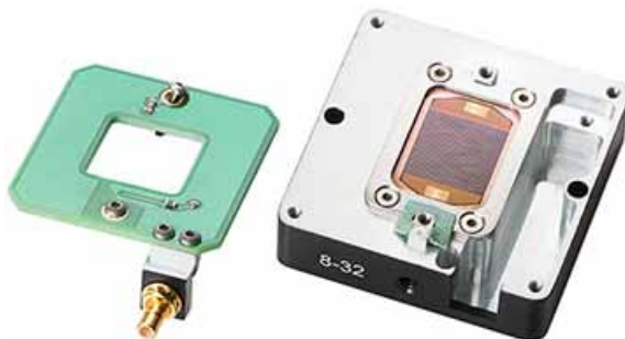
Figure 3-13. Pass-Thru Circuit Board—Ready to Install
