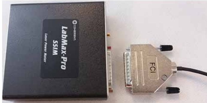
Figure 2-16. Connect the Sensor to the Meter
