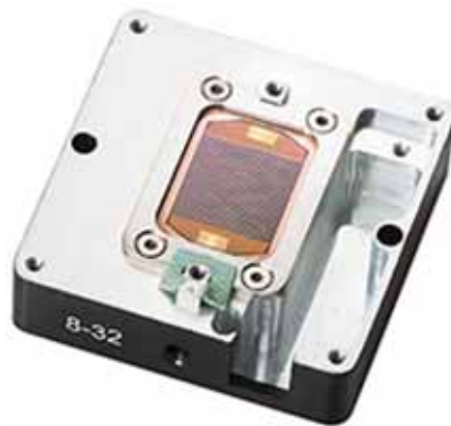
Figure 3-28. Retention Frame Secured
