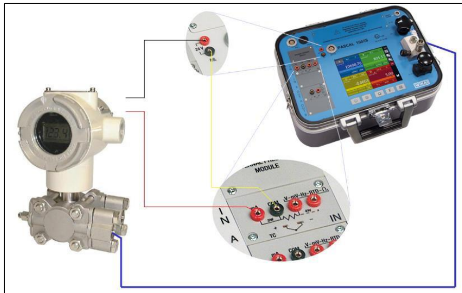
Figure 106 – Pressure transmitter calibration example
