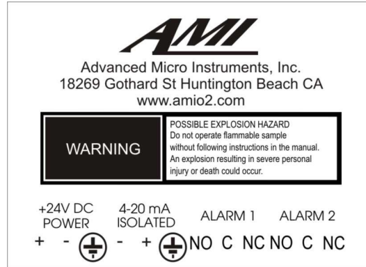
Figure 2. Back panel of the 201LC.
