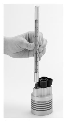
Figure 4 Inserting thermometer
