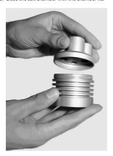
9. Fasten the salt chamber on the holder in the base plate and close the measurement holes with rubber plugs.
