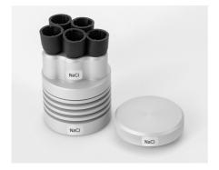
11. Allow approximately 24 hours for stabilization before use so that the salt solution reaches the equilibrium humidity.
