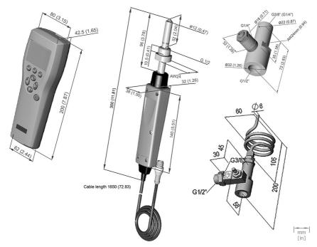
Figure 30 Dimensions of MI70 indicator, DMP74 probe, DSC74 sampling cell, and DSC74C sampling cell (left to right and top to bottom)
