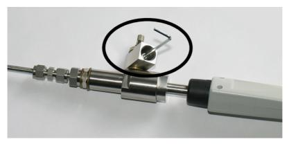
Figure 27 Removing the leak screw
