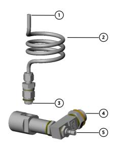
Figure 19 Alternative assembly of DSC74C for tight spaces
