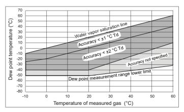
Figure 28 DMP74A dew point accuracy vs. measurement conditions
