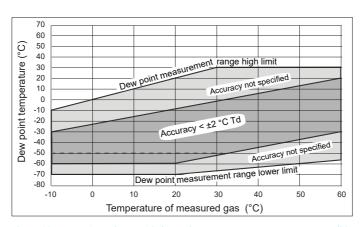
Figure 29 DMP74B and DMP74C dew point accuracy vs. measurement conditions
