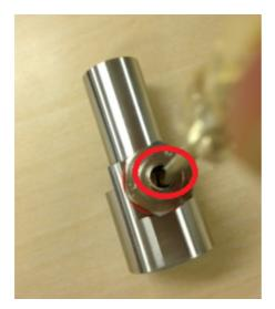
Figure 21 Turning sampling cell valve screw with flathead screwdriver
