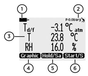
Figure 4 DM70 basic display
