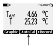
Figure 11 Hold/Save replaced by AutoCal
