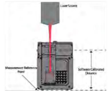
Calibrated beam path for precise focus spot location
