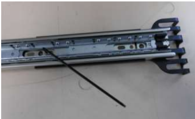
Figure 100 – Attach Rack Mount Adaptors to Outer Slides
