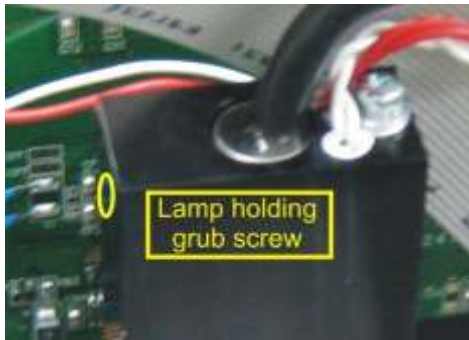
Figure 95 – Location of UV Lamp Fastening Grub Screw
