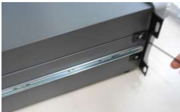
Figure 99 – Rack Mount Ears Fitted to Analyser
