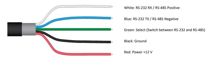
The Green wire should be connected to Ground to enable RS-485 communication, or it should be connected to 12 V power for RS-232 communication. Text for the White and Blue wires above refers to the port that the wires should be connected to.
