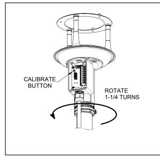
Fig 4.2.1 Orientation of Wind Sensor Using Electronic Compass
