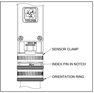
Fig 4.2.3 Proper Engagement of Orientation Ring with Sensor
