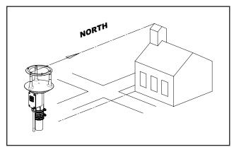
Fig 4.2.2 Sighting of Wind Sensor using Geographic Feature
